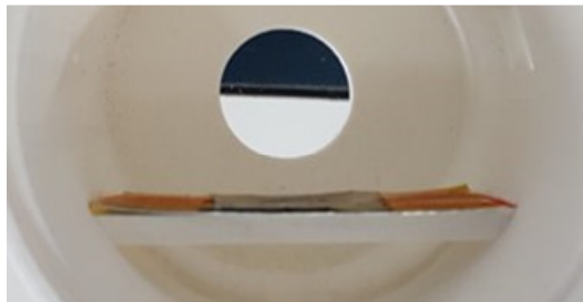
Figure 3.16 SAW device fixed in a flat position inside a breath chamber for the detection of respiratory rate and apnoea
