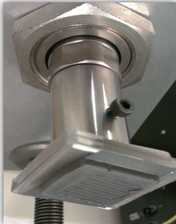
Figure 4.13: a patterned PDMS stamp attached to the actuator of the electric cylinder.
