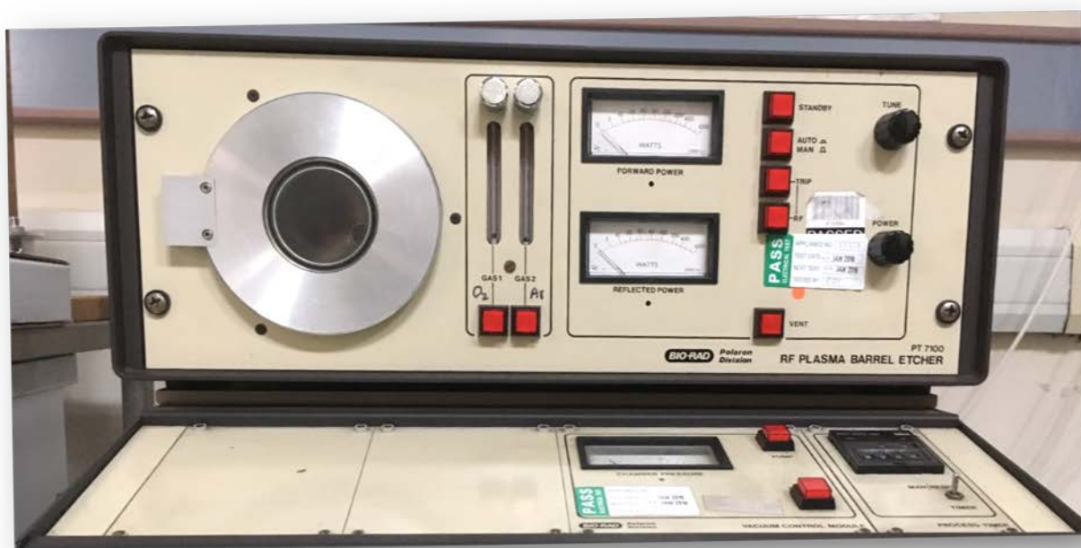
Figure 3. 11: PT 7100 RF Plasma Barrel Etcher that was used in this research for treating the surface of the substrates.
