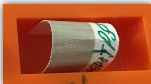
Figure 6.27: photograph of smooth bending test set up on the IJP PEDOT:PSS.
