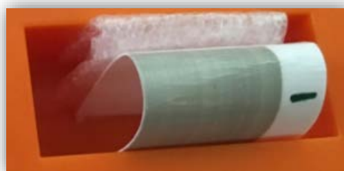
Figure 6.29: photograph of sharp bending test set up on the IJP PEDOT:PSS.
