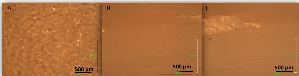
Figure 6.25: optical microscopic images of the ceramic coated paper in flat state (a) and bending state; smooth (b) and sharp (c).
