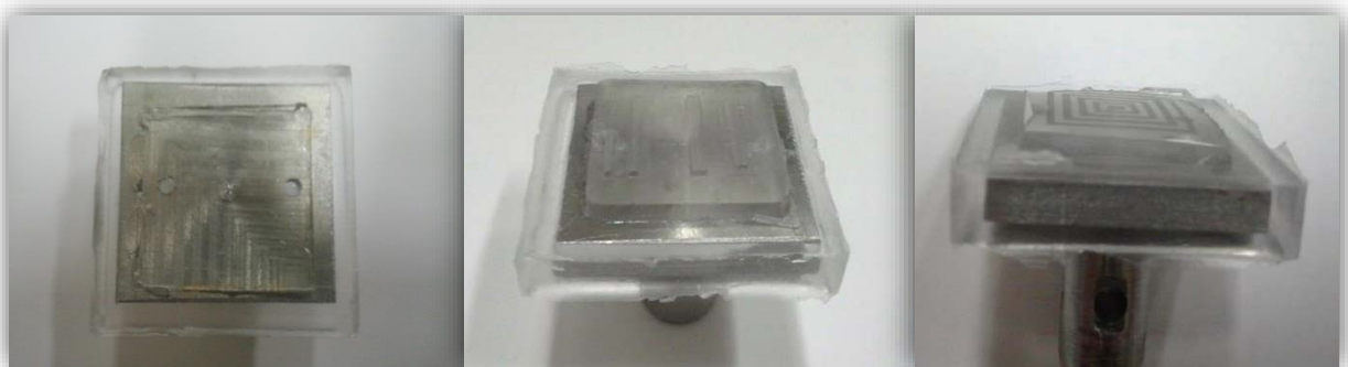
Figure 4.5: some of the PDMS stamps that were cast with some masters for purpose of testing the stamp printing machine.
