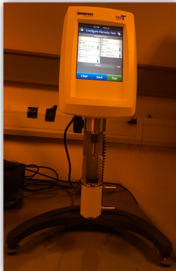
Figure 3.10: the viscometer that was used in this research for measuring the viscosity of the liquids of interest.
