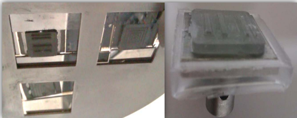
Figure 4.11: some of the PDMS stamps after (Al) deposition.
