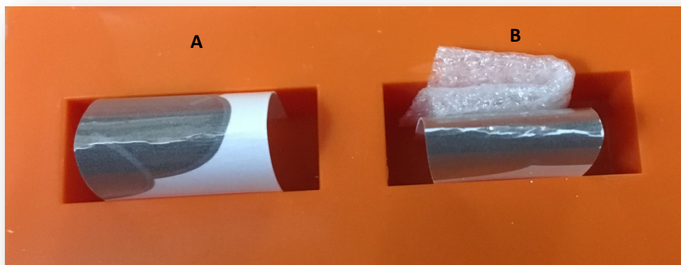
Figure 6.18: photograph of smooth (a) and sharp (b) bending of the IJP silver.
