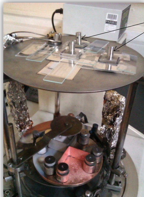
Figure 4.10: PDMS stamps inside the thermal evaporator for (Al) deposition.
