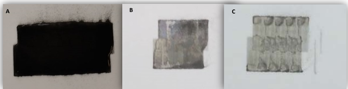
Figure 6.38: photographs of inkjet printed graphene oxide on PEL paper; a) 3 layers, b) 2 layers and c) 1 layer.
