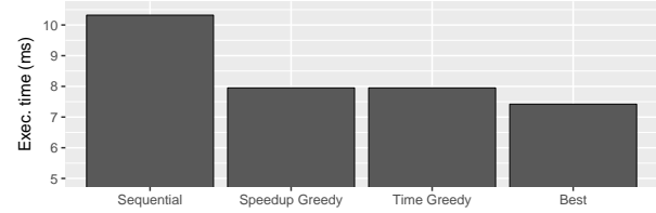
Figure 1. Execution time to run the five kernels from Table 1 using different scheduling strategies.
