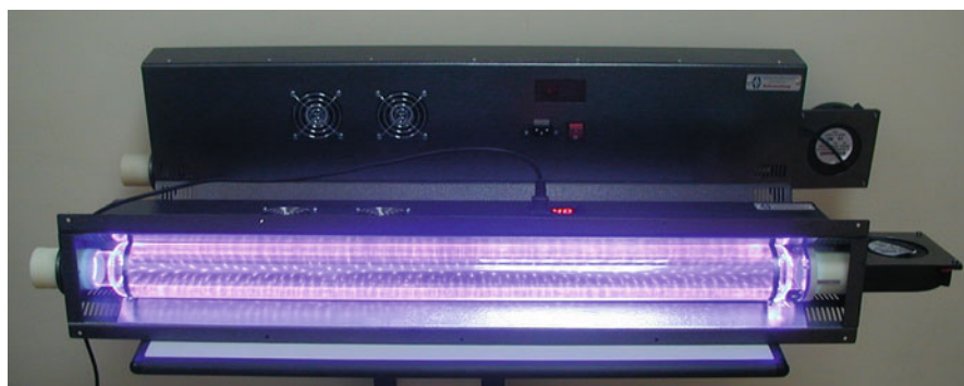
Fig. 19.2 General view of KrCl- and XeBr-excimer lamps (BD_X model)
