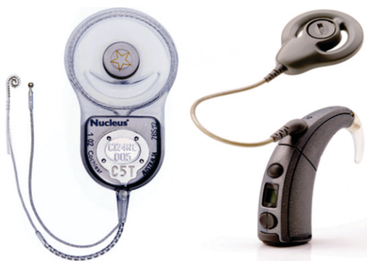
Fig. 1 : Cochlear implant-internal and external components
