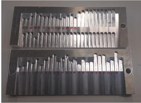
Figure 8. Workpiece after experimentally defined stability lobe diagram
