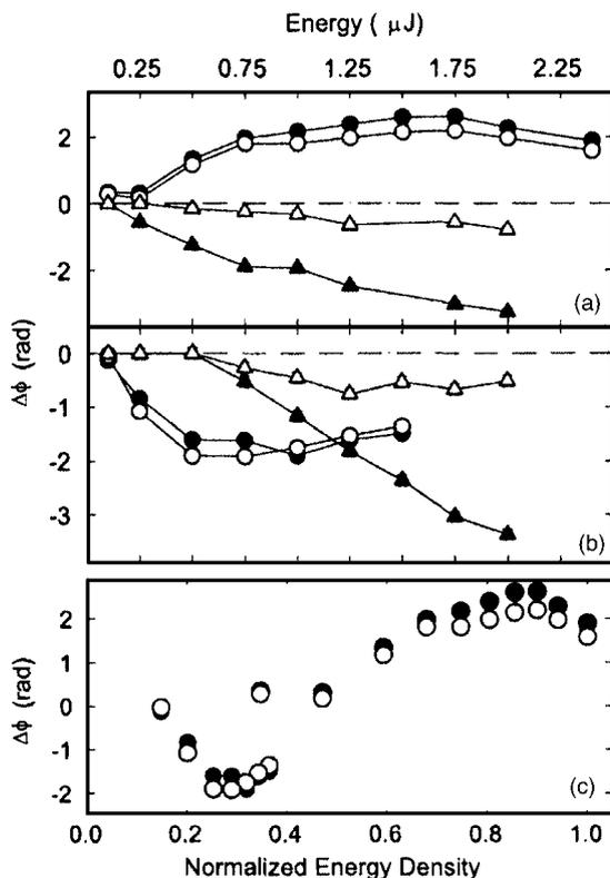
FIG. 2. Phase shift, for polarization parallel (filled marks) and orthogonal (open marks) to the polarization of the writing laser, due to laser-induced refractive index changes in glass (triangles) and  $\text{SnO}_2$  containing glass (circles), at (a) high-NA and (b) low-NA focusing of the writing beam vs the laser pulse energy. (c) Phase shift in glassceramics vs the estimated relative value of maximum energy density per pulse along the propagation axis inside the material.
