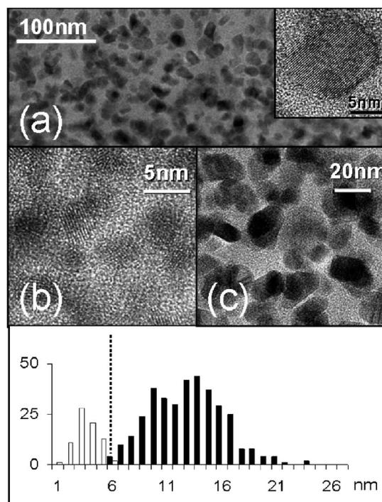
FIG. 4. (a) TEM image of  $\text{SnO}_2$  nanoparticles in 16 mol %  $\text{SnO}_2$ : $\text{SiO}_2$  glass ceramic. Inset: High resolution TEM image of a  $\text{SnO}_2$  nanoparticle. (b) Reduced-size and (c) unperturbed-size nanoparticles in laser-processed and -unprocessed regions, respectively, of the material. Histogram: statistics of cluster sizes from sampling of laser-modified (white bars) and unmodified (black bars) regions.
