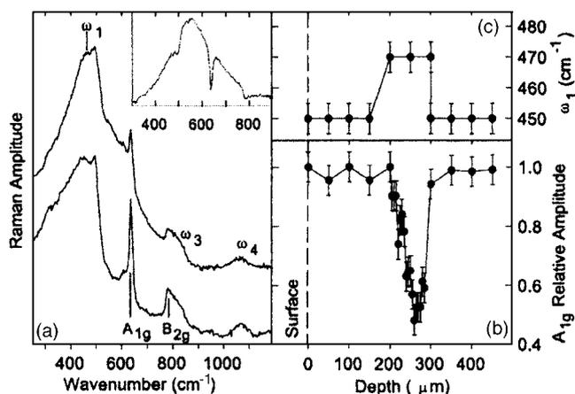
FIG. 3. (a) Confocal micro-Raman spectra at 50 (lower curve) and 250  $\mu\text{m}$  (upper curve) from the sample surface after femtosecond writing at 1.25  $\mu\text{J}$  of energy pulse. Inset: difference spectrum. (b) Amplitude decrease of the  $A_{1g}$  mode of crystalline  $\text{SnO}_2$  and (c) energy of the  $\omega_1$  silica mode at increasing depth from the front surface of the material.
