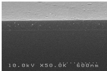
FIG. 1. SEM image of a pink sample (type 1): etched cross section (magnification: 50000 $\times$ , tilt angle: 10 $^\circ$ ). The gold nanoparticles can be seen as white spots randomly distributed in the 130-nm-thick sol-gel glass film.
