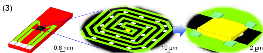
Figure S4 Transfer and deposition of the wedge on the MEMS chip.
