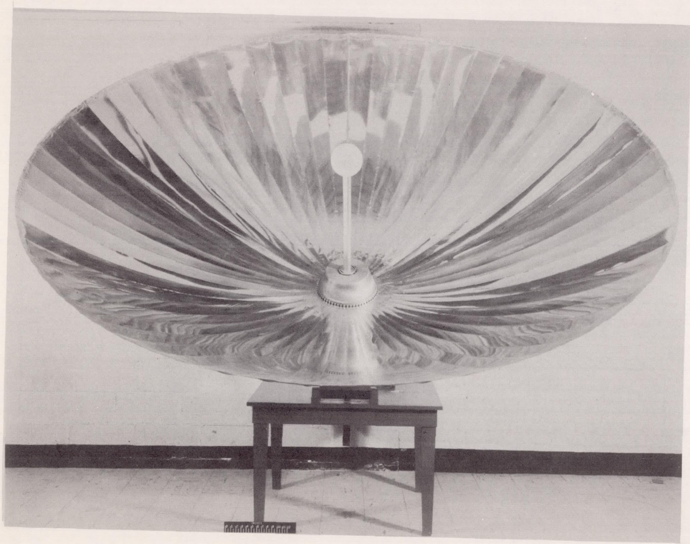
Figure 3.- The 10-foot-diameter concentrator after being heated.
