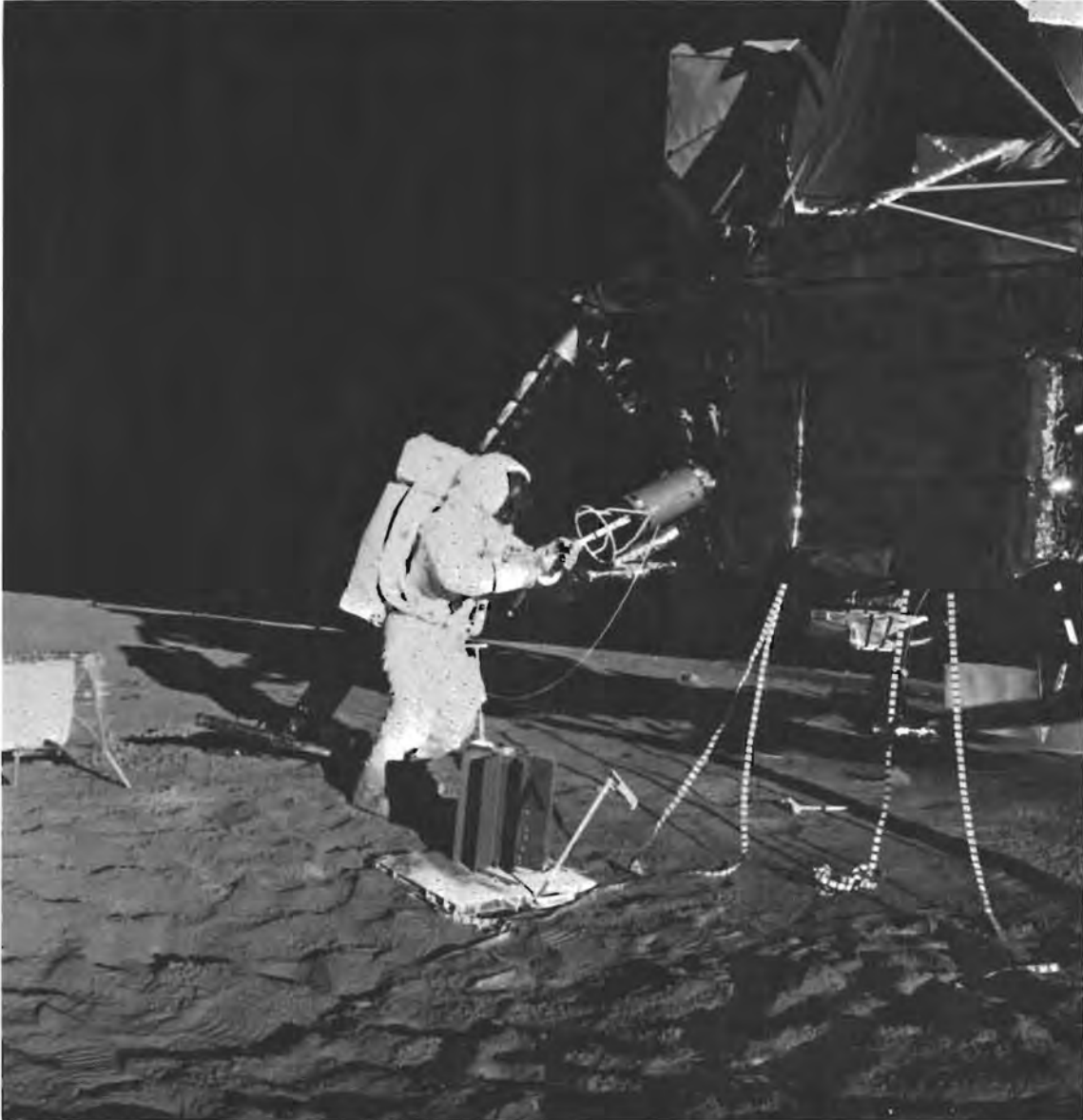
Figure 9-3.- Lunar Module Pilot extracting the fuel cask. The radioisotope thermoelectric generator is shown near the crewman.
