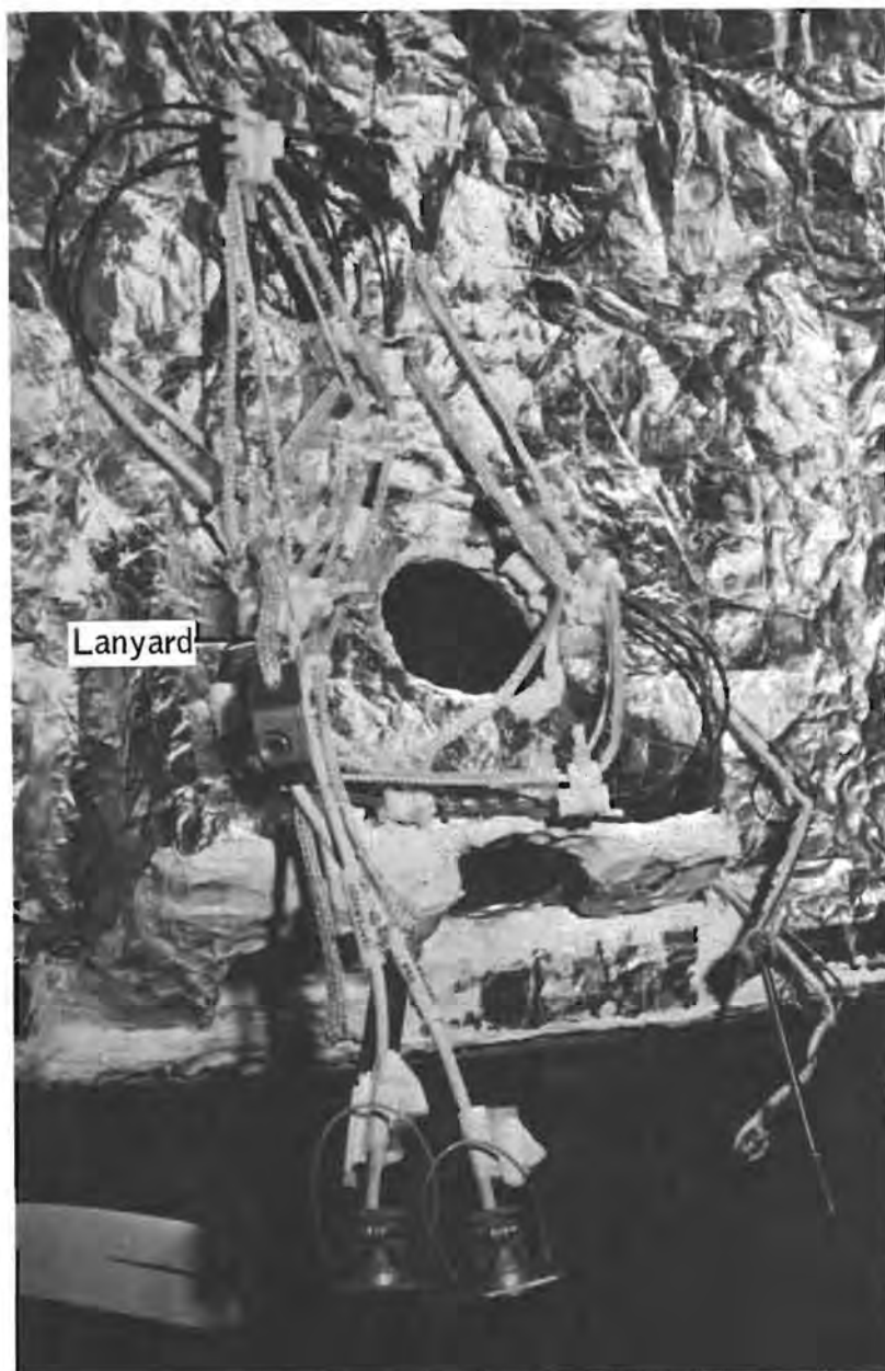
Figure 14-18.- Forward heat shield mortar umbilical.
