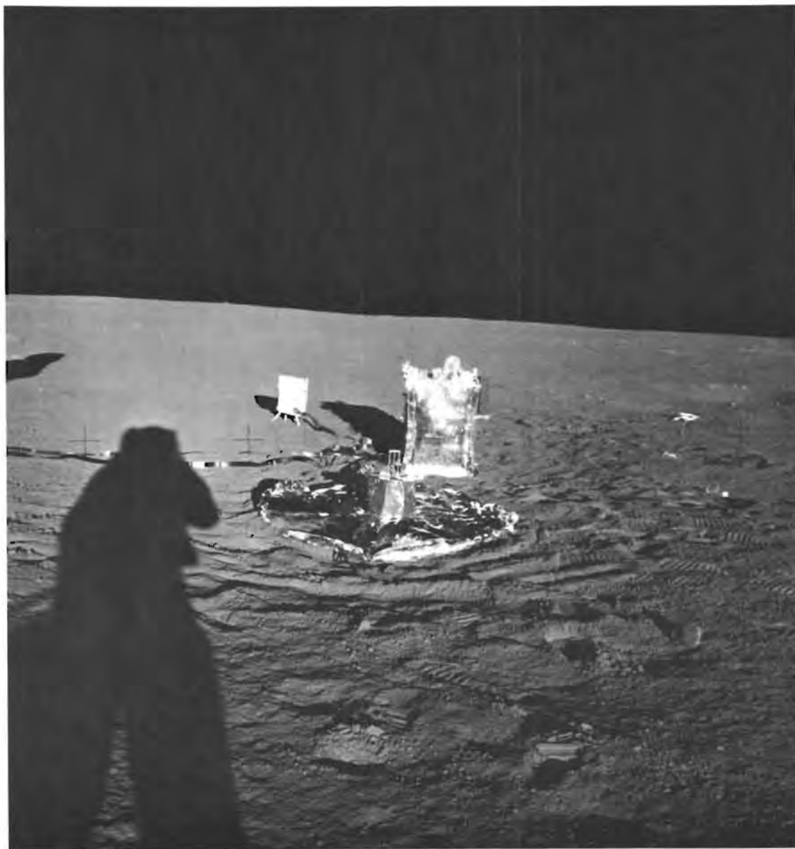
Figure 3-5.- Passive seismic experiment and the experiment central station in the foreground with the undeployed suprathermal ion detector experiment in the background.
