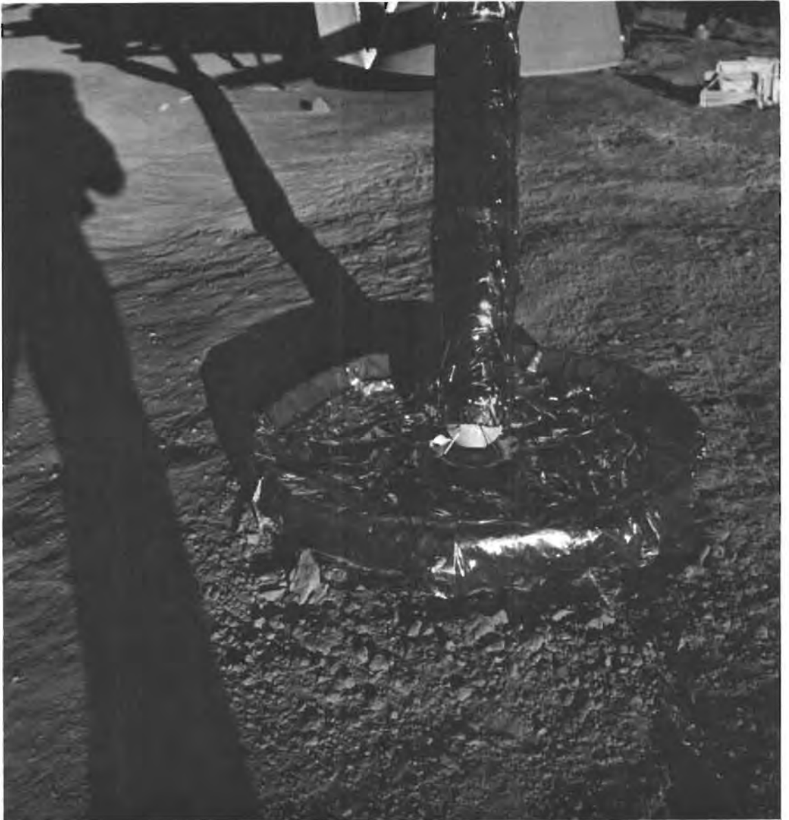
Figure 3-22.- Detail of lunar module minus Z footpad showing disturbance of fine-grained material as viewed from the east.
