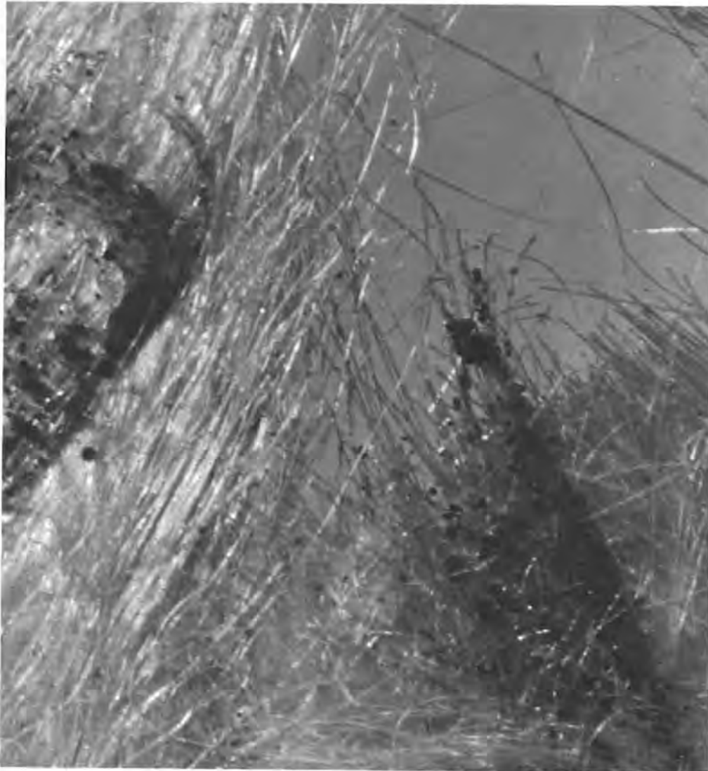
Figure 14-19.- Deposit on end of heat shield lanyard.
