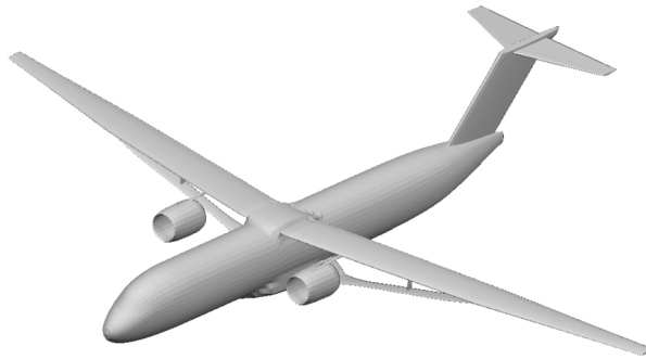
Figure 2 VSPAERO Model of TTBW
