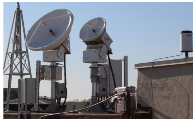
Beacon Receivers, Disdrometer, and Weather Station at the POLIMI DEIB Building
