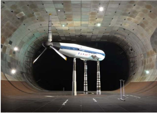
Figure 1. TTR/699 installed in the USAF NFAC 40-by-80-Foot Wind Tunnel (45-deg yaw).
