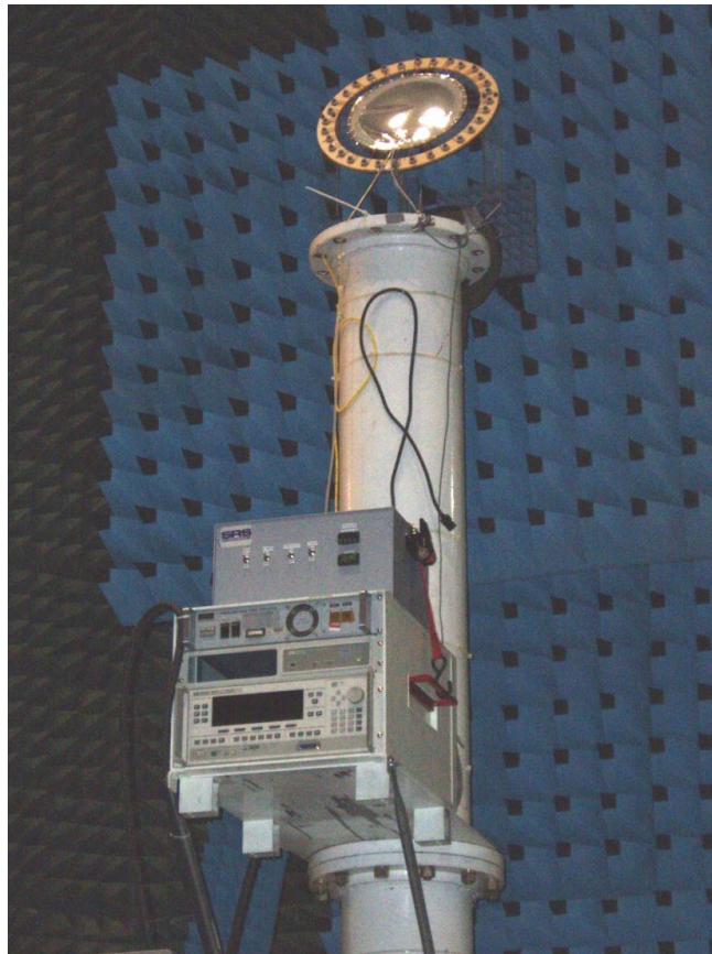
FIGURE 2: 0.3 Meter Antenna in GRC Planar Near-Field Antenna Test Facility
