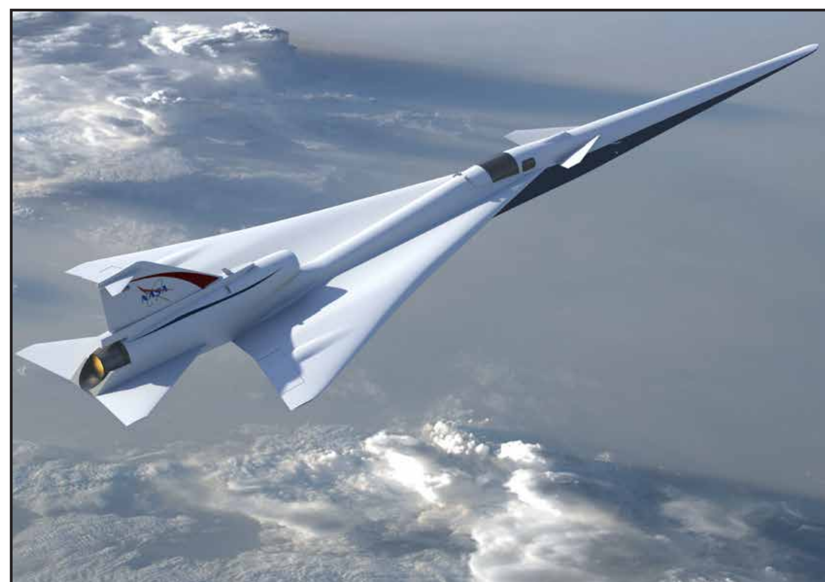
Illustration of NASA's planned Low-Boom Flight Demonstrator aircraft. The close proximity of the tail cone surfaces and jet motivated the work of jet surface interaction noise prediction (for example, jet scrubbing noise) with the use of hybrid Reynolds-averaged Navier Stokes/Large-Eddy Simulation methods. NASA, Lockheed Martin
