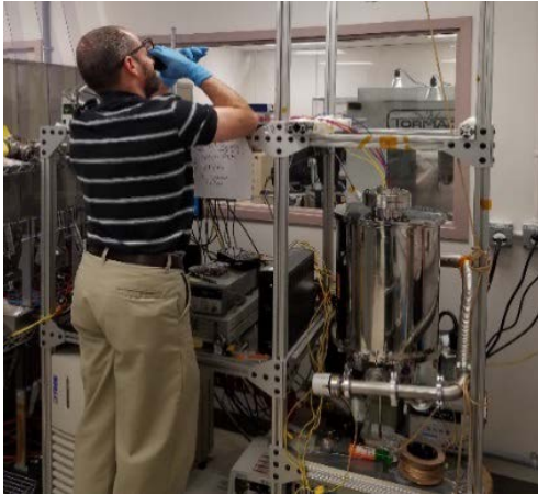
Figure 14: Alejandro Rodriguez-Perez sets up the PER data logging system with custom fiber optic thermal vacuum feedthroughs produced by the Photonics Group.
