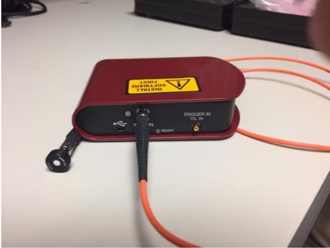
Figure 55: Spectrometer used for xenon calibration
