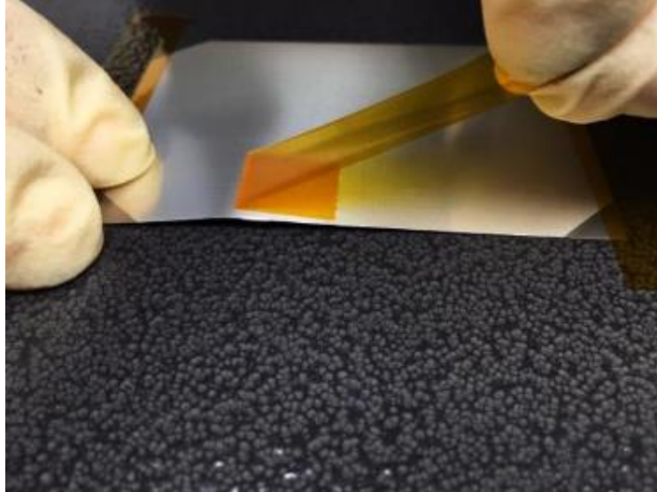
Figure 4: Tape Pull Test on Concentrator
