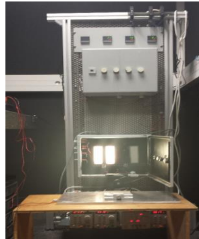
Fig. 5. Experimental bench of OLED aging tests (overview)
