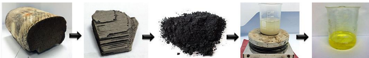
Figure 5.1: Recovery of precious metals (Pd(II), Pt(II) and Rh(III)) from the spent catalytic converter.
