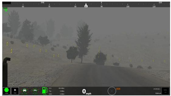
Figure 1.6: Go/NoGo Driving Aid showing terrain slope
