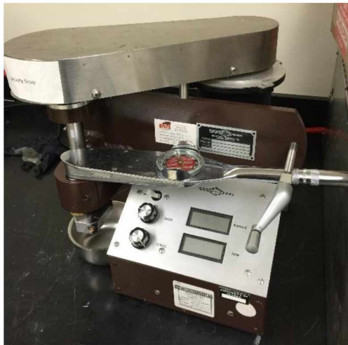
(c) OFITE EP and Lubricity Tester
