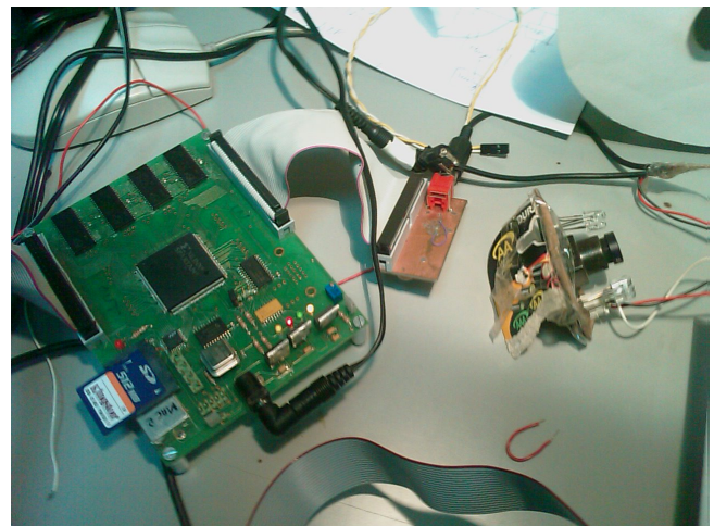
Figure 3. Synthetic retina boards
