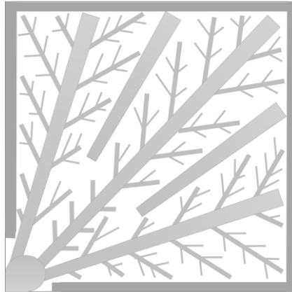
Figure 6. Interdigitated Flow Field design based on tree-like structures, by Ouellette et al [98].
