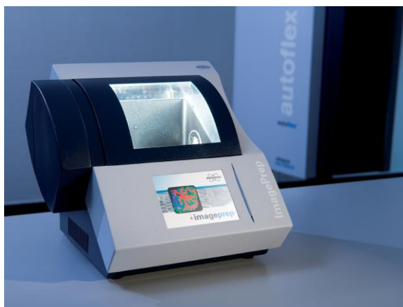
Figure 2.2: The ImagePrep™ station for matrix deposition. (Image from ImagePrep Manual) 16
