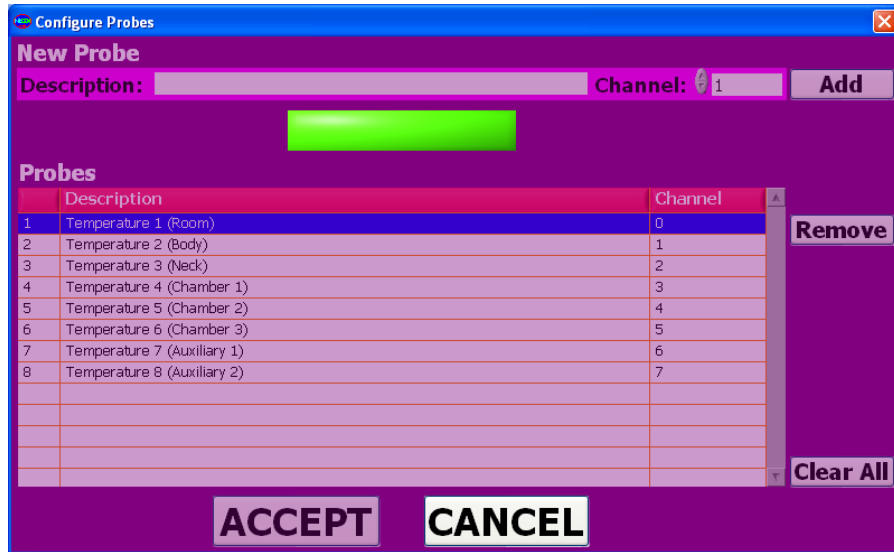
Figure 37: Temperature probe locations. Note that these settings cannot be changed by the user. However, there are two “Auxiliary” temperature probe channels that the user can assign as they find necessary. Notes on the location of these probes may be added to the test settings notes or otherwise recorded by the user.
