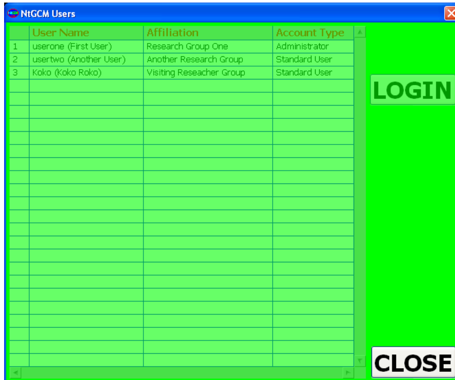
Figure 27: List All Users dialog when there is a user already logged in. New user selection and login functions are disabled
