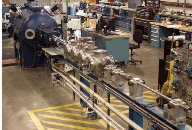
Fig. 3. WSTF 4.3 mm two-stage light-gas launcher.
