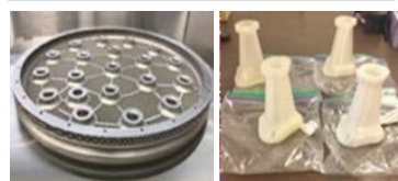
ISM Design Database Development Life Support Systems Retaining Plate (Left); Logistics Reduction Urine Funnels (Right)
