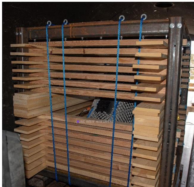
Figure 6 Overall front oblique view of sample. Image taken with the wood blast mitigation measures in place, the larger gap present between the slats, provides an avenue for the projectile to pass through to the target. Dyneema rope was also employed to bind the wood to the steel structure.
