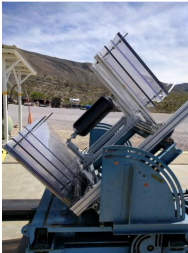
Figure 4 Representative of test fixture that would secure COPV tank types 1, 4 and 5 (typical).
