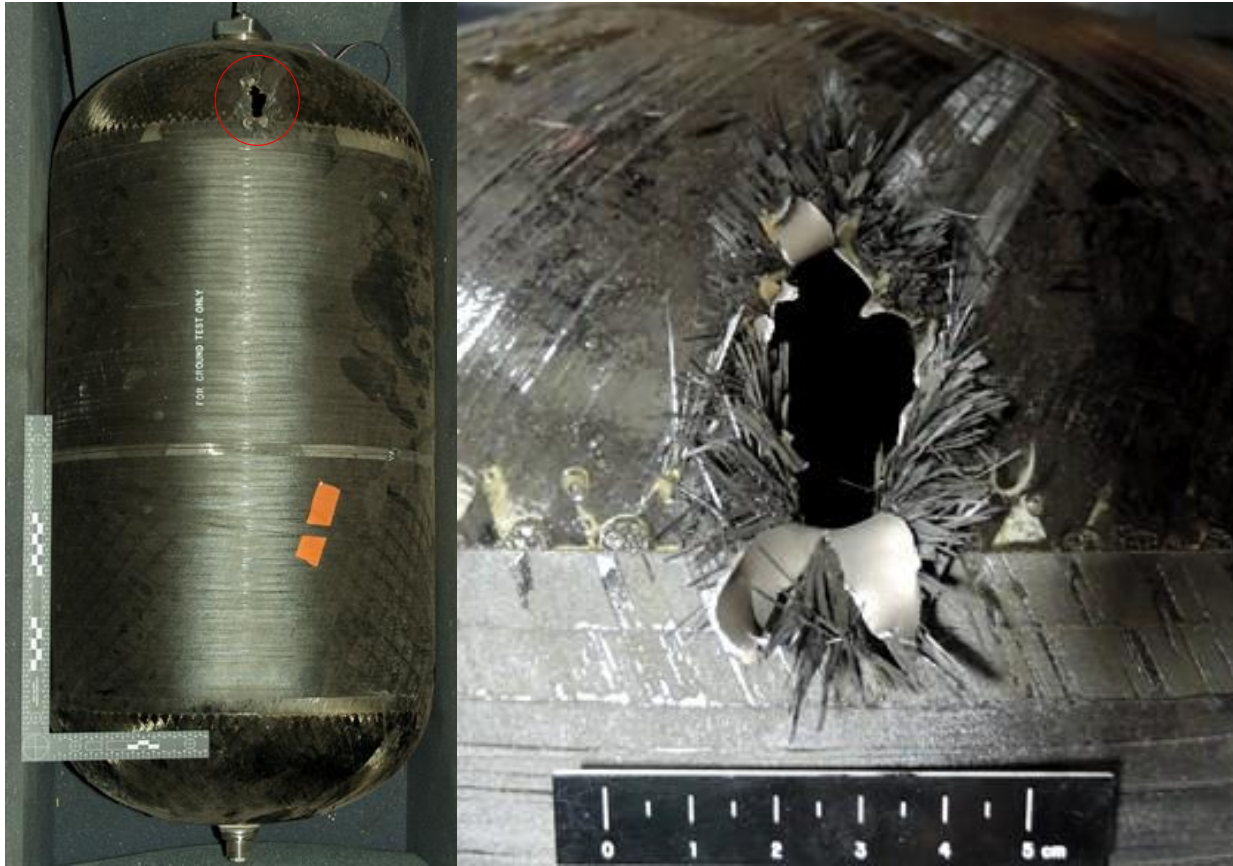
Figure 11 Overall view of damage to COPV tank (left) and overall view of entry damage (right / damage located within red circle in adjacent image) for HITF17082.
