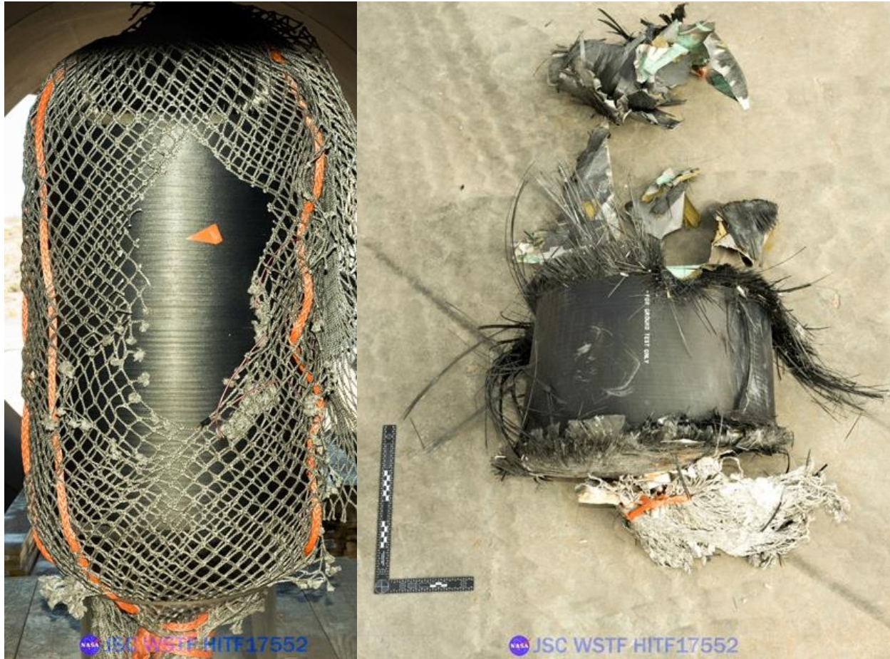
Figure 15 Overall front view of target within the target tank pre-test (left) and overall view of most significant COPV tank carcass remnants post-test HITF17552 on pad outside of target tank (right).
