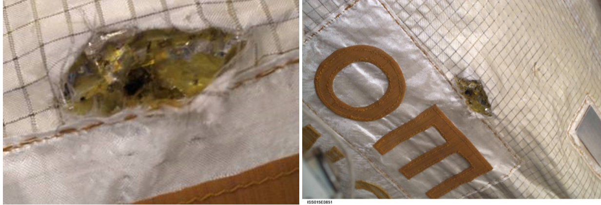
Fig. 16. FGB compressor thermal blanket MMOD damage.
