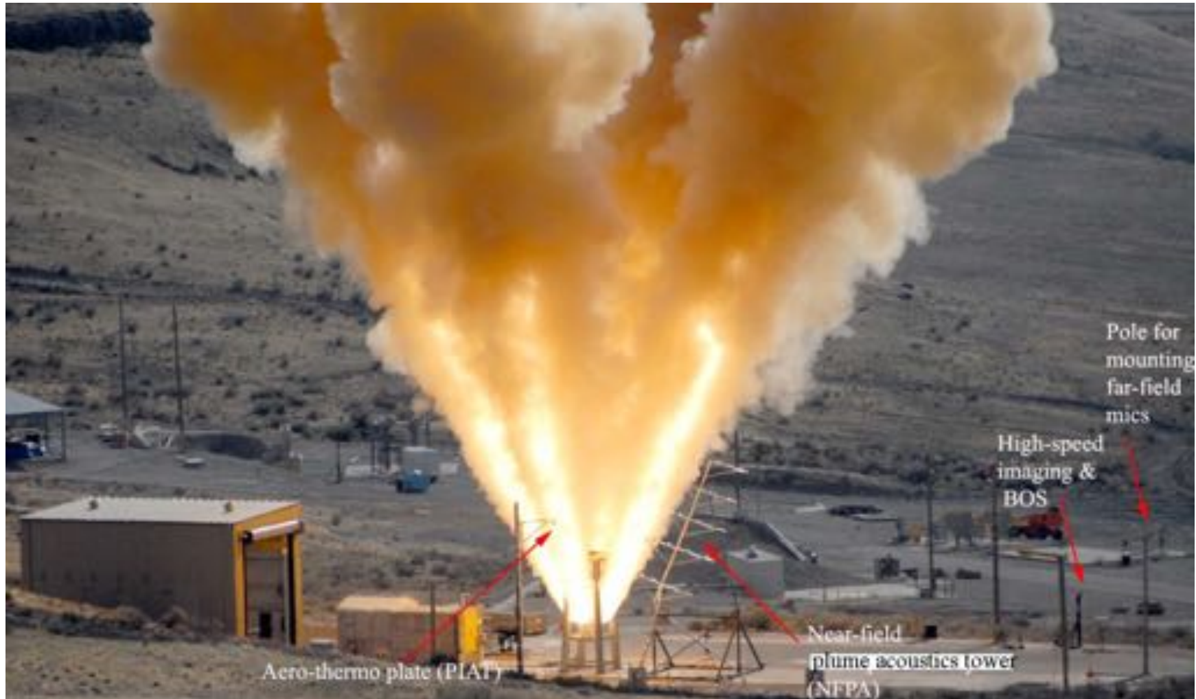
Picture from ST1 abort motor ground test
