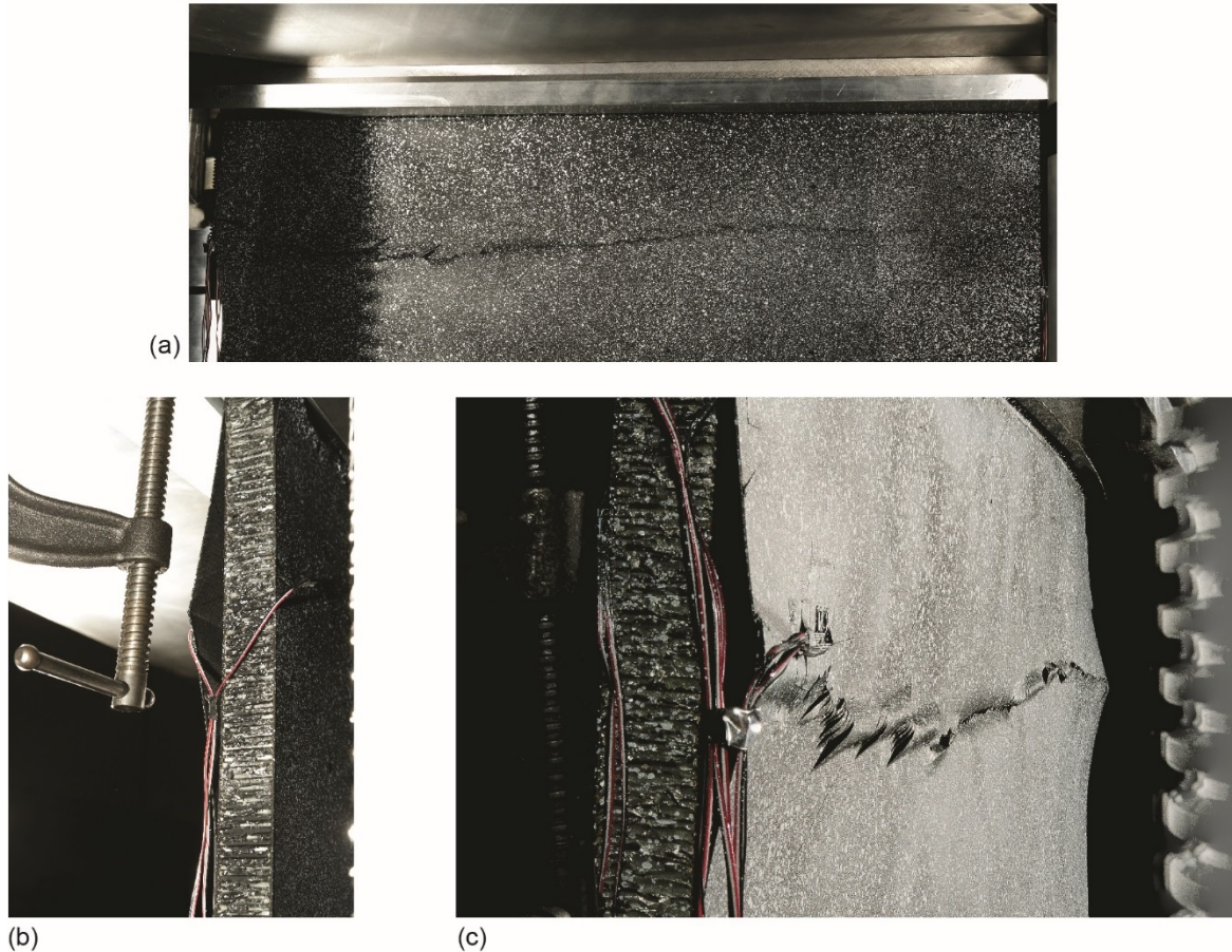
Figure 9.—Failure mechanisms observed after catastrophic failure of panel immediately after onset of buckling. (a) Facesheet cracking. (b) Facesheet core disbonding. (c) Facesheet buckling, cracking, and core disbanding.
