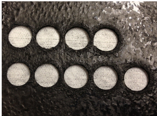
SEM specimens cut with different laser power/speeds
