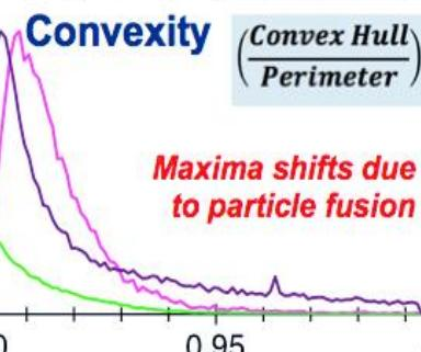
Maxima shifts due to particle fusion
