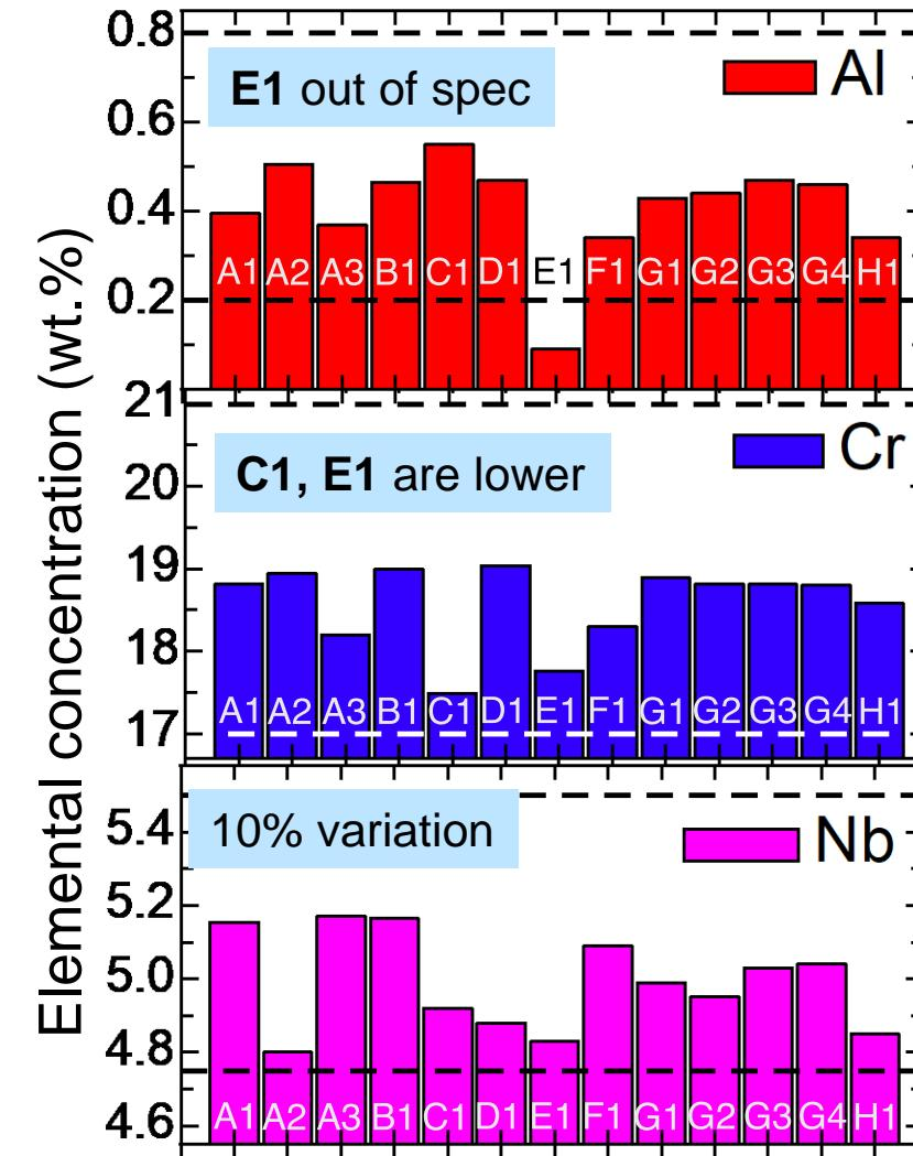
High **trace impurity** could lead to segregation, inclusions, & weldability issues
