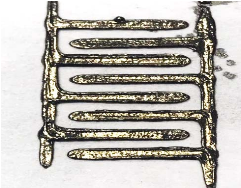
3D-Printed Al-Fe 3 O 2 Nanothermite Sintered CO 2 Sensor
