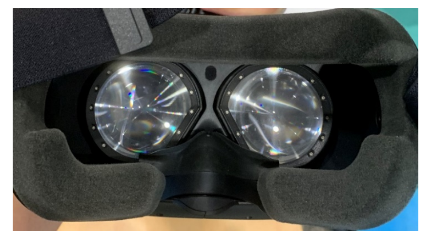
Embedded eye-tracking in VR goggles
