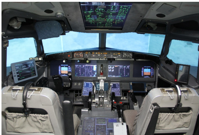
Figure 12. Flight simulator with TAP v2 on the Captain's EFB. Photo by M. Cover.
