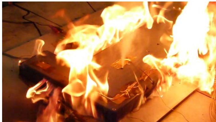
Figure 1 - Catastrophic Failure of the Initial Battery A Design (18)
