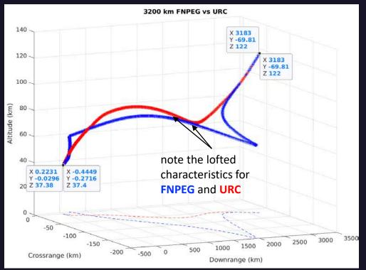
\*Comparable profiles between the two algorithms are observed,  $\leq$ 3km miss distance is desired
