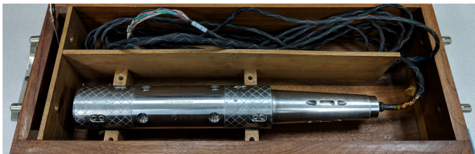
Fig. 1 NASA's 2.5 inch diameter MK34A six-component force balance.
