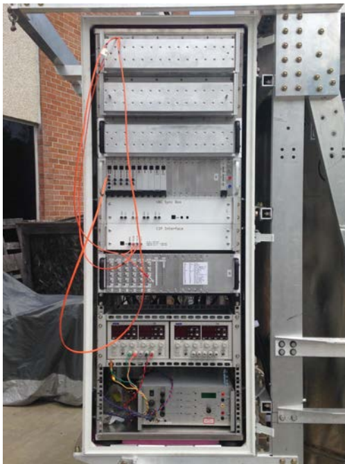
(a) Starboard 30U box mounted on payload with subracks visible.
