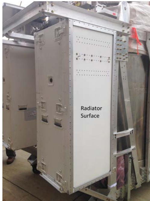
Fig. 7 Starboard 30U box with radiator panel and conductive bar attachment bolt patterns.
