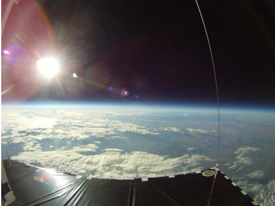
Fig. 13 Earth shield position during flight with relatively large field of view to Earth and relatively small Sun visibility.
