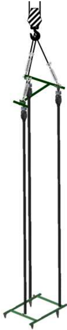
Fig. 11 The full ground vibration test soft-support system with three bungees.
