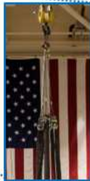
Modified Three Bungee Suspension System without Spreader Bar
