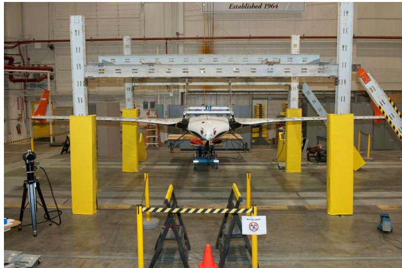
Fig. 22 The X-56A Multi-Utility Technology Testbed in moment of inertia testing configuration.
