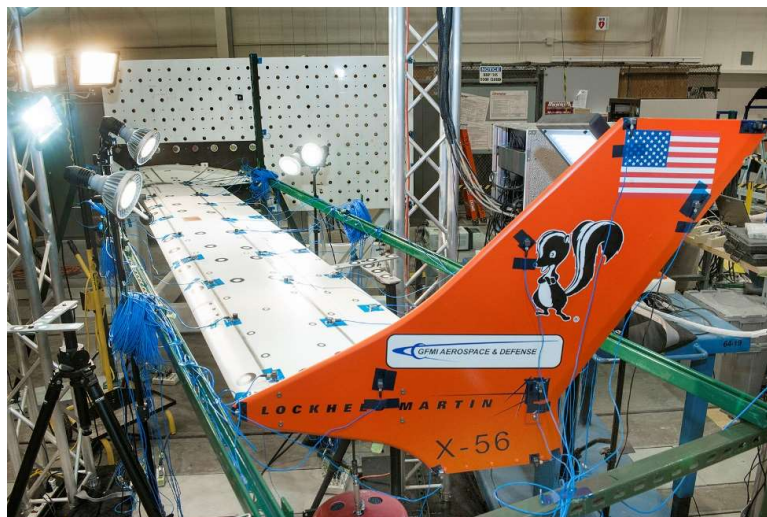
Fig. 3 The left wing strongback ground vibration test.
