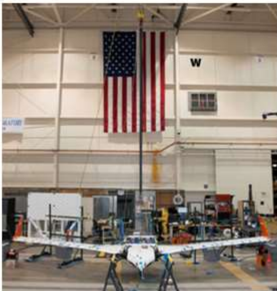
Fig. 15 Configuration changes to the bungee soft-support.
