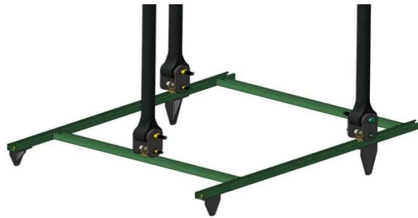
Fig. 13 The ground vibration test soft-support system connected to the lifting frame by three bungees.
