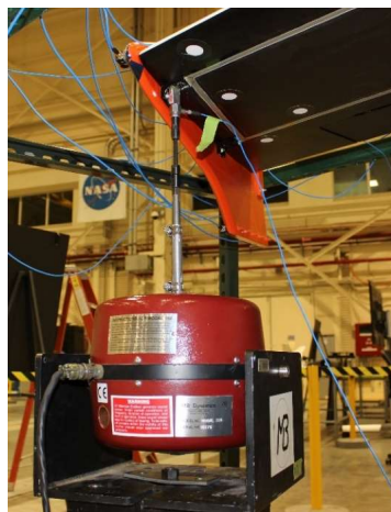
Fig. 9 The location of the leading-edge spar shaker on the right wingtip.
