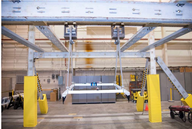
Fig. 21 Front view of the lifting frame in the moment of inertia testing configuration.
