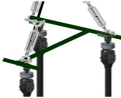
Fig. 12 The ground vibration test soft-support system connected to the upper spreader bar by three bungees.
