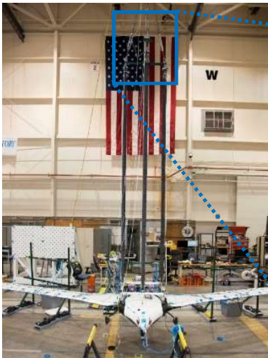
Original Three Bungee Suspension System with Spreader Bar
