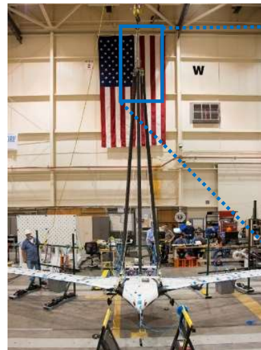
Modified Three Bungee Suspension System without Spreader Bar
