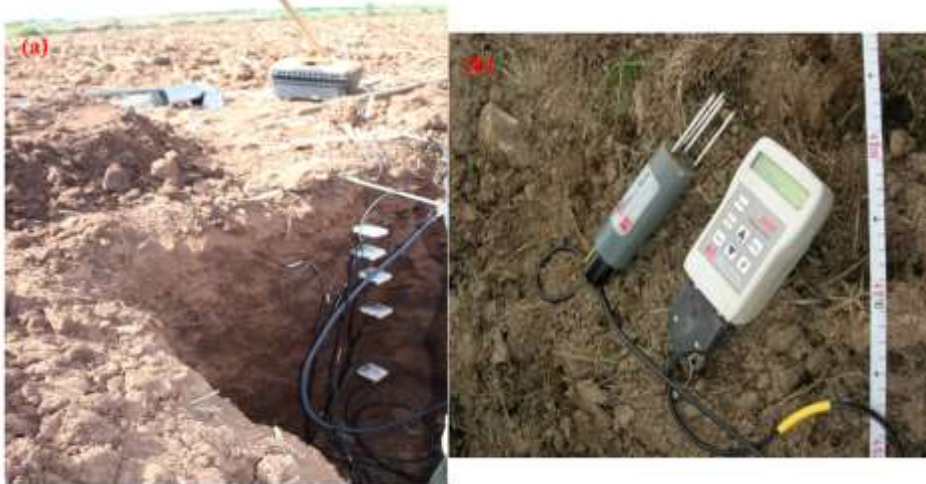
Figure III. 4. Photograph of (a) TDR (Time Domain Reflectometry) and (b) Theta Probe instruments
