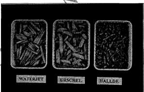
Fig. 4 Apple strips cut by the waterjet, Urschel and Hällde cutting system
