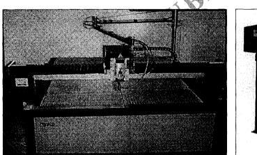
Fig. 1 Waterjet cutting system of Digital Contol
