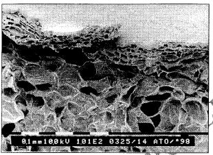
Fig. 12 SEM picture just uner the peel of an apple strip, cut by the Hällde cutting system.
