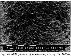
Fig. 16 SEM picture of mushroom, cut by the Hällde cutting system
