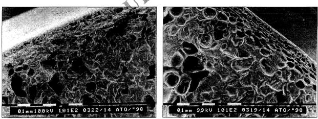
Fig. 10 SEM picture just under the peel of an apple strip, cut by the waterjet cutting system
