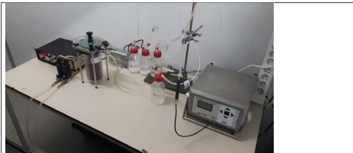
Figure 2-8: PHGA test setup for kiwifruit: a pump draws air through a \text{KMnO}_4 filled cuvette and feeds mass flow controllers flushing each one of two 550l containers filled with kiwifruits. Measurements were done on the air expelled from the containers. Also visible are the gas wash bottles with saturated salt solutions equilibrating at 1^\circ\text{C} to create various levels of Relative Humidity.
