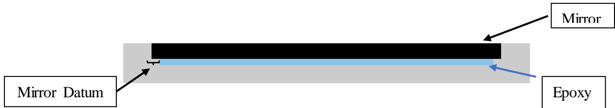
Figure 11. Mirror Mounting Concept Design, Epoxy Recession
