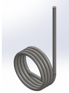
Figure 36. Top Mirror Hinge Assembly: Spring
