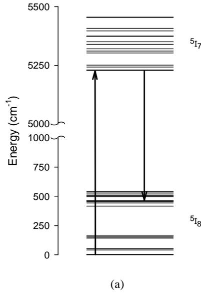
Fig. 2. (a) Ho:YAG energy level diagram for the in-band pumped 2.1micron transition<sup>5</sup>.
