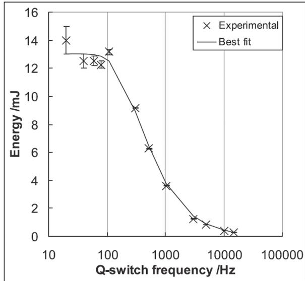
Fig. 6. Ho:YAG pulse energy as a function of repetition rate at the maximum available thulium-laser pump power of 68W.
