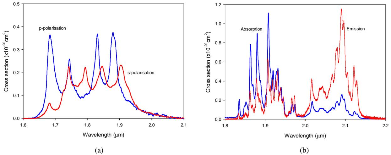
Fig. 1. (a) Room temperature Tm:YLF polarized emission cross-section versus wavelength after<sup>4</sup>, (b) Room-temperature Ho:YAG measured absorption cross-section and calculated emission cross section via the reciprocity method<sup>4</sup>.
