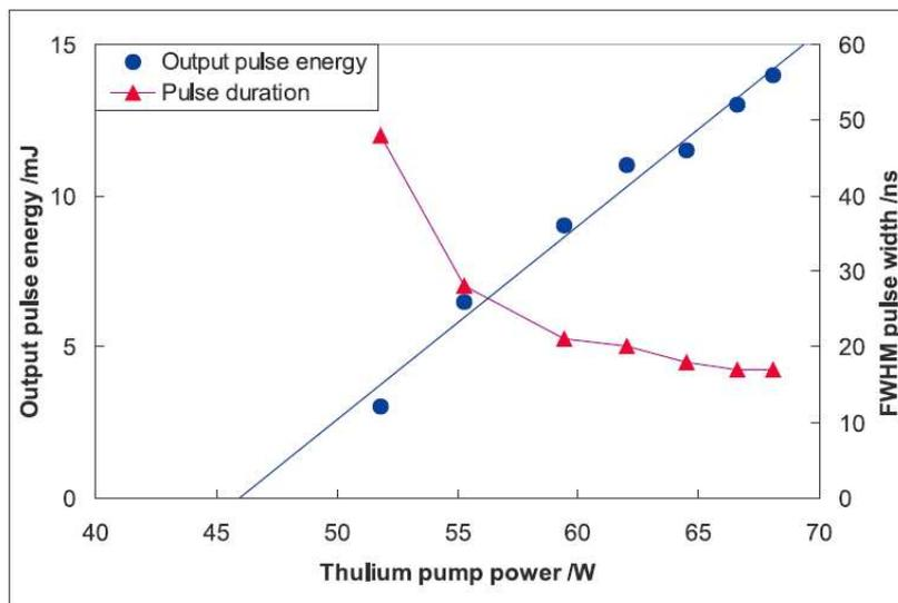
Fig. 5. Ho:YAG QS laser performance at a 20Hz repetition-rate.
