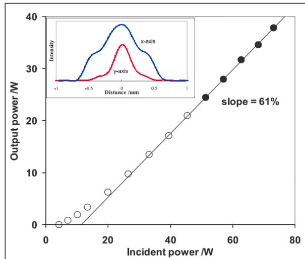
Fig. 4. Ho:YAG rod laser performance pumped by two spatially-multiplexed diode-pumped Tm:YLF slab lasers. Insert represents the mode profile in the laser rod.
