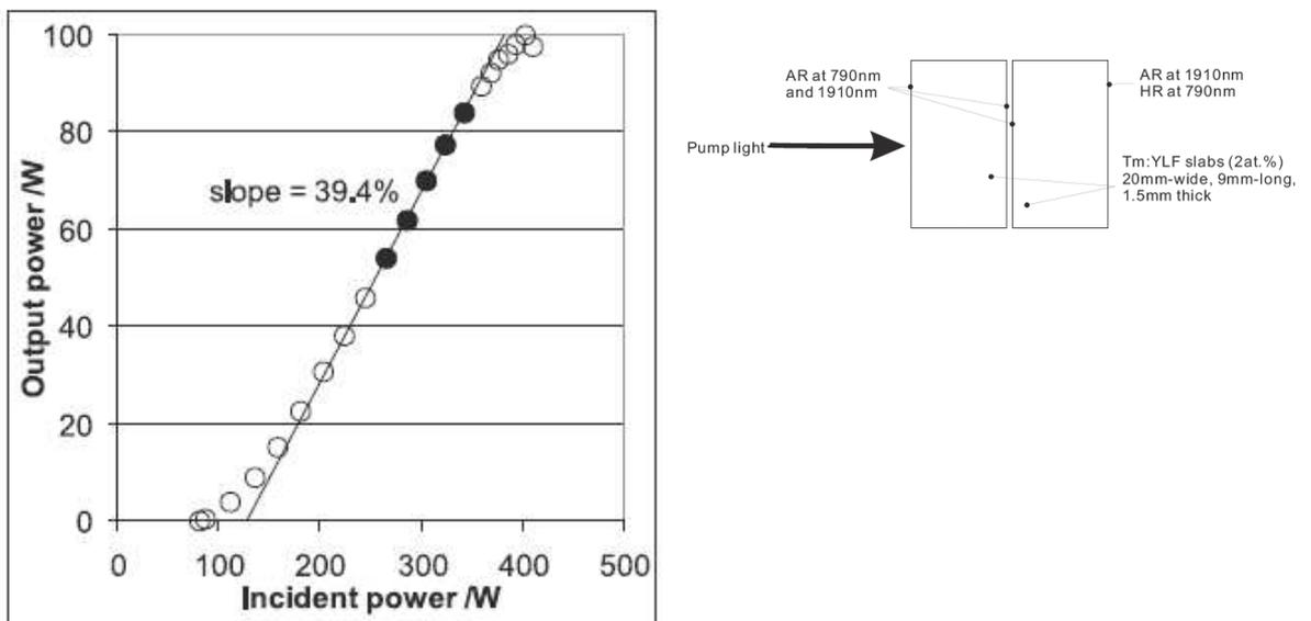
Fig. 7. Laser performance with the Tm:YLF dual slab gain block, illustrated in the inset.
