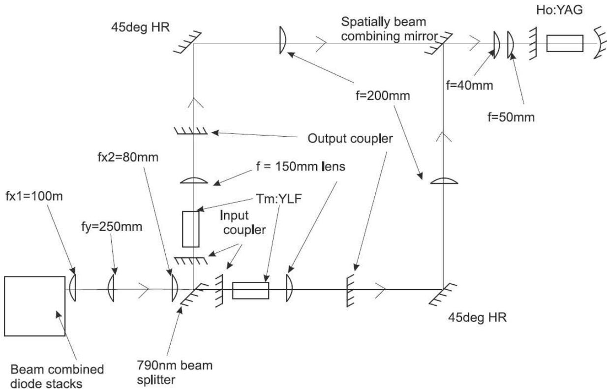
Fig. 3. Experiment layout for the diode-pumped Tm:YLF slab lasers, spatially multiplexed to end-pump a Ho:YAG rod laser, in the CW configuration. Note for the QS configuration two YAG Brewster plates and an RTP Pockels cell were inserted into the cavity between the output coupler and the Ho:YAG rod.
