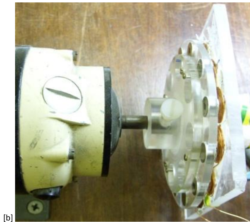
Figure 7.2 Rotor (a) and motor test rig (b).
