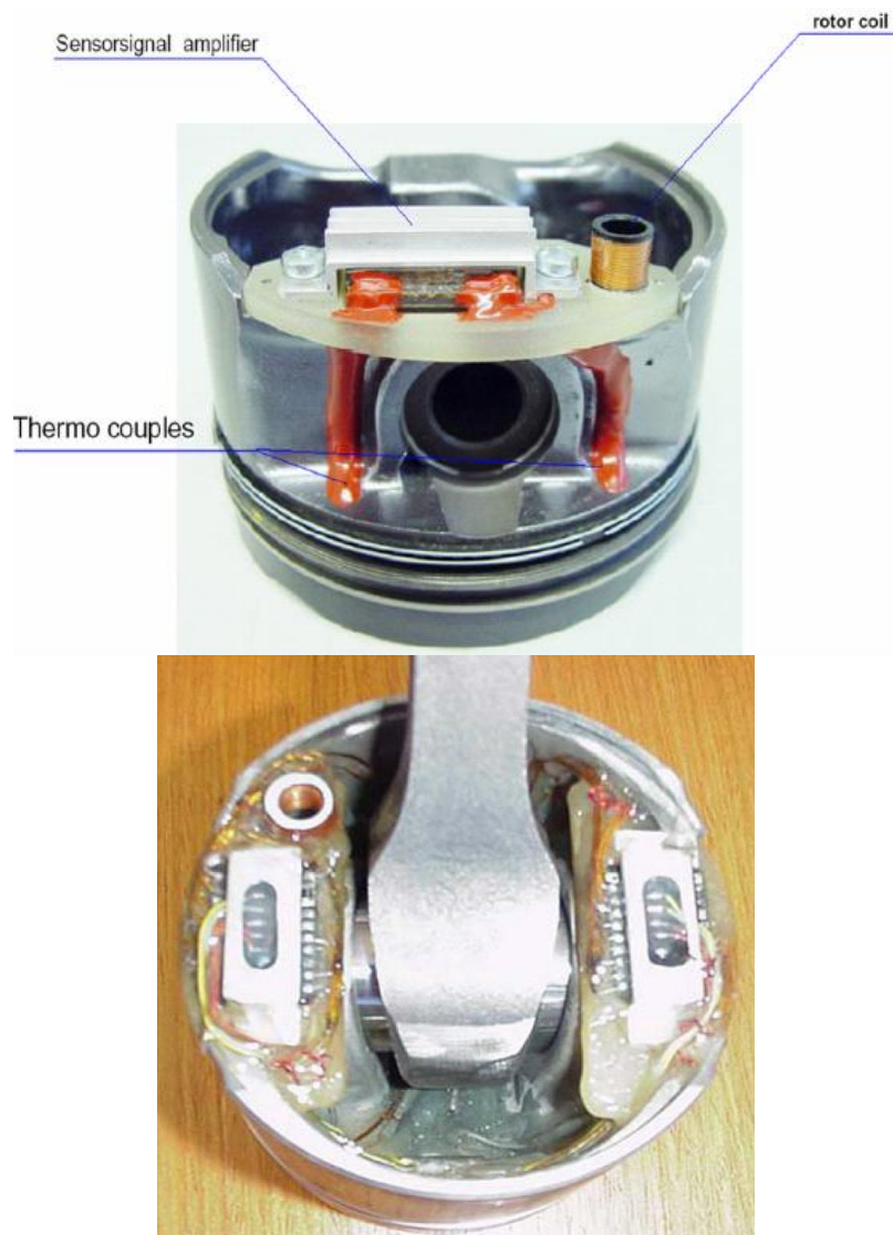
Figure 3.8 Location of components [104].
