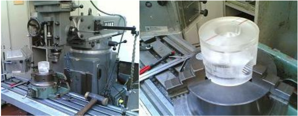
Figure 3.18 Machining of the Prototype acrylic piston block.
