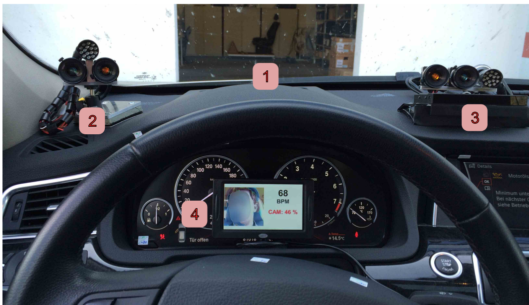
Figure 57: Camera-based measurement setup in the car environment: (1) Dashboard, (2) Daylight and NIR camera with illumination at the A-pillar, (3) Daylight and NIR camera with illumination at the dashboard's center, (4) Display for instant feedback on the HR measurement. The application of cbPPG in the car environment was investigated in cooperation with the Alps Electric Europe GmbH.
