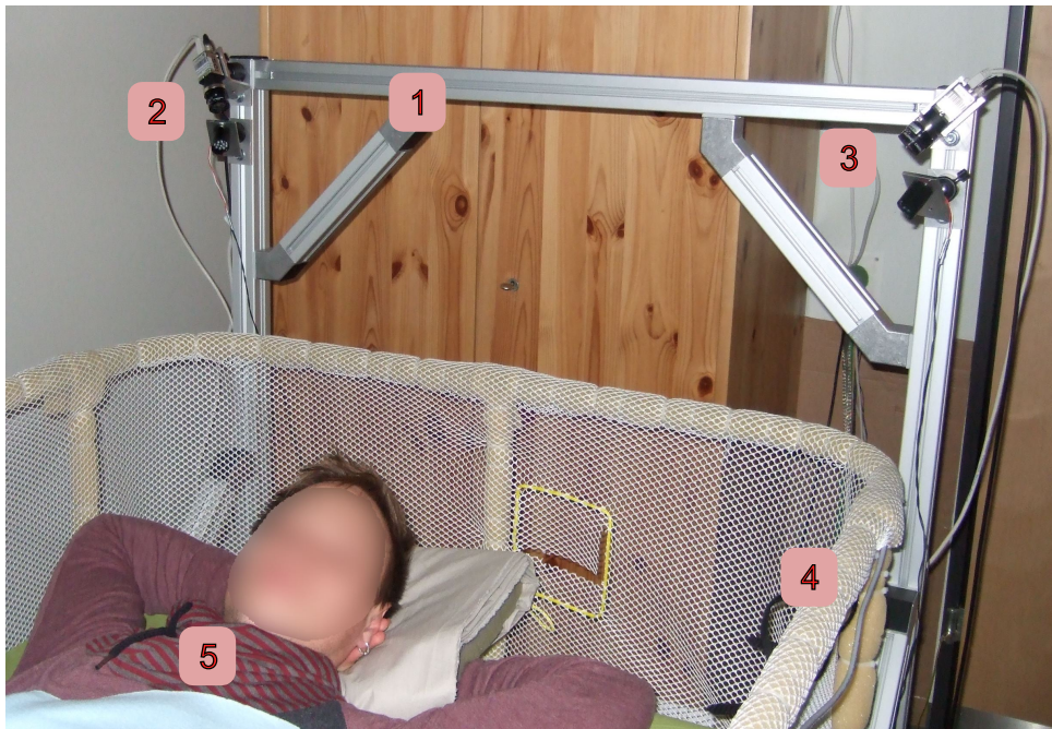
Figure 56: Camera-based measurement setup in the sleep laboratory: (1) Constructional framework, (2) Camera and NIR illumination at the left bed side, (3) Camera and NIR illumination at the right bed side, (4) Test bed, (5) Test subject. The application of cbPPG during sleep was investigated in cooperation with the Institute of Robotics and Intelligent Systems at the ETH Zürich.
